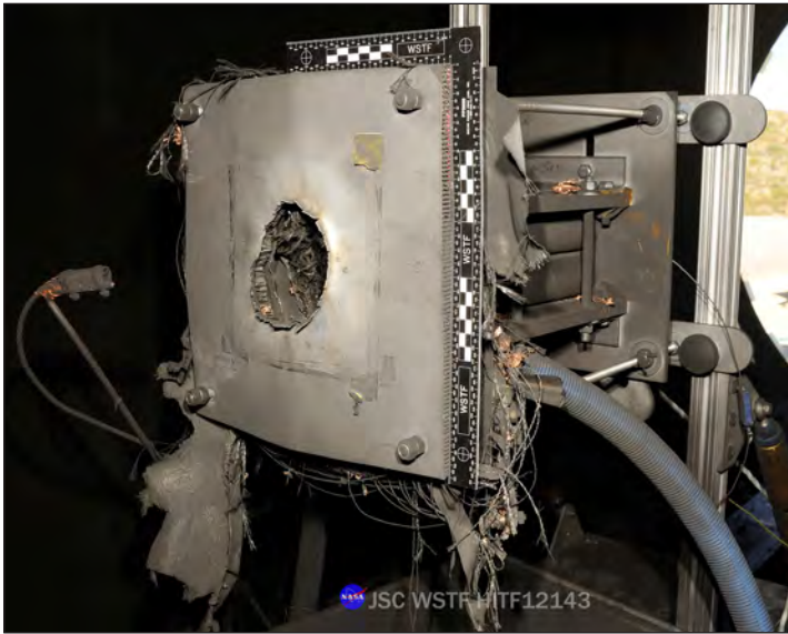
Figure 2. After test imagery of shield protecting the Li-ion battery with a large 10-cm-diameter hole burned through the aluminum honeycomb panel.
