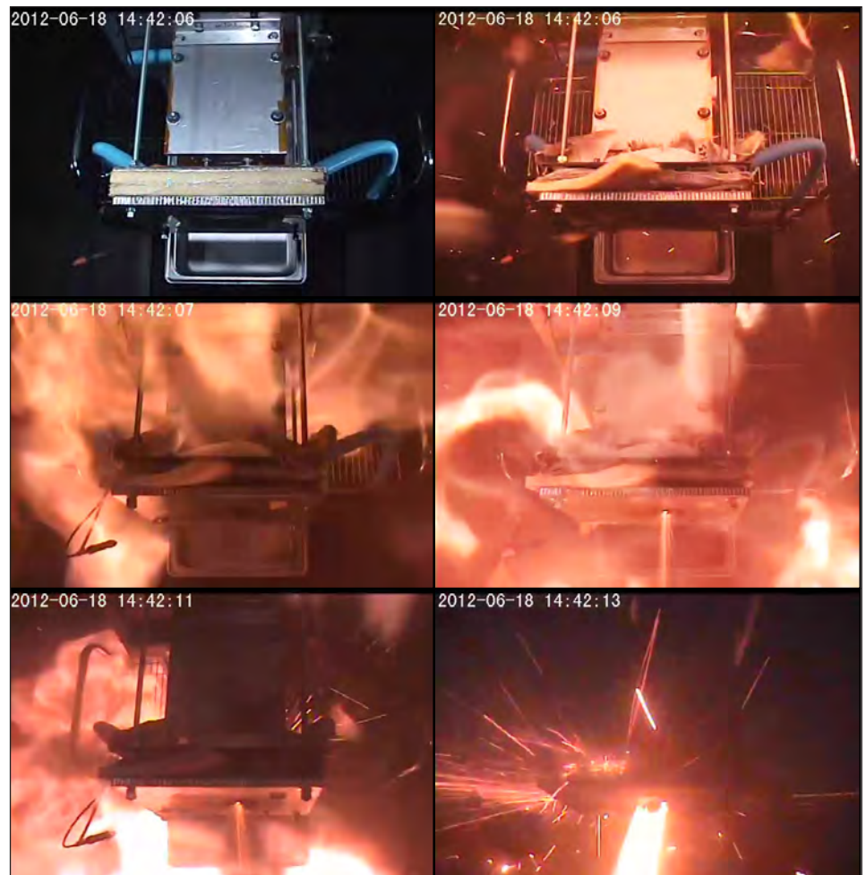
Figure 1. Sequence from video (1-2 seconds between frames) of hypervelocity impact test HITF-12143 on a Li-ion battery cell.
