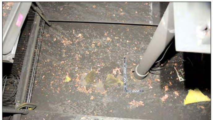
Figure 4. Chamber floor after HITF-12143 showing a large number of metal fragments were ejected from the cell. Note the black and white checker-board pattern in the L-shaped ruler at the bottom of the chamber. Each block in the checker-board is 1 cm in length.
