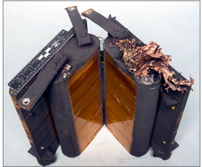
Figure 3. The two Li-ion cells from HITF-12143 showing material ejected from cell interior of the impacted cell (on right), and little damage to the neighboring cell (on left) that remained operational after the test.
