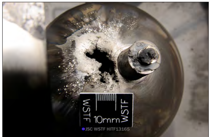
Figure 5. ISS Ni-H 2 cell hypervelocity test damage/perforations (on the left) Test HITF13144, 5.0-mm aluminum spherical projectile at 6.66 km/s and (on the right) HITF13165, 3.8-mm steel spherical projectile at 6.87 km/s.
