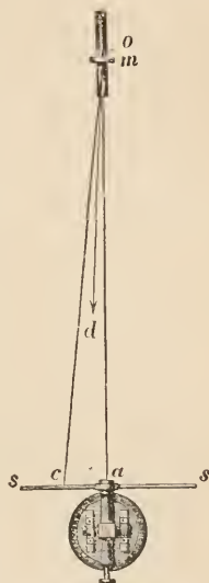
FIG. 19. MEASUREMENT OF SMALL ANGLES OF DEFLECTION WITH MIRROR AND LENS.
