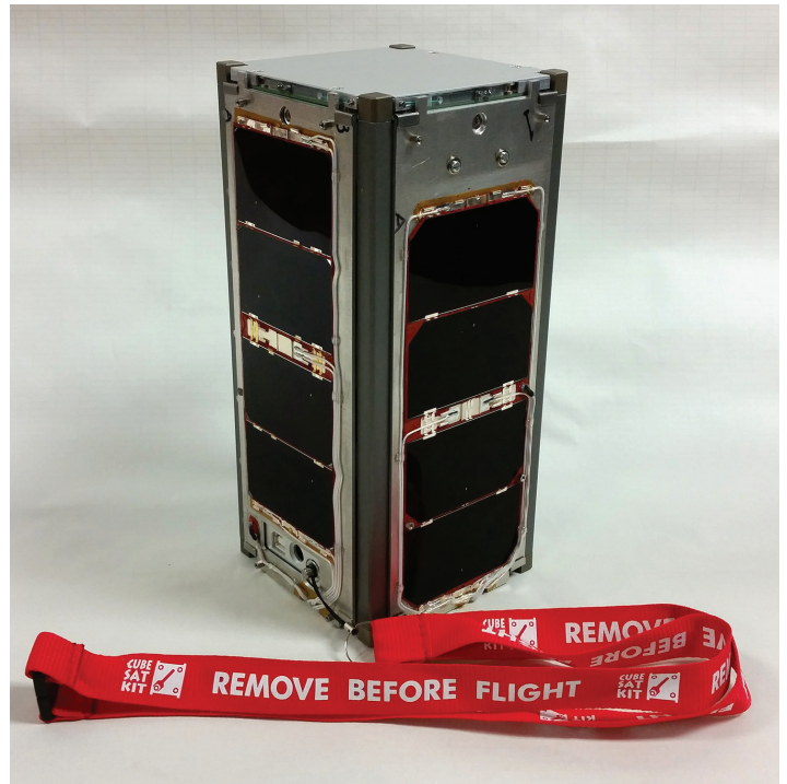
The standard CubeSat size uses a "one unit" or "1U" measuring 10x10x10 centimeters and is extendable to larger sizes; 1.5, 2, 3, 6, and even 12U. A CubeSat typically weighs less than 2 kilograms (4.4 pounds) per unit.
