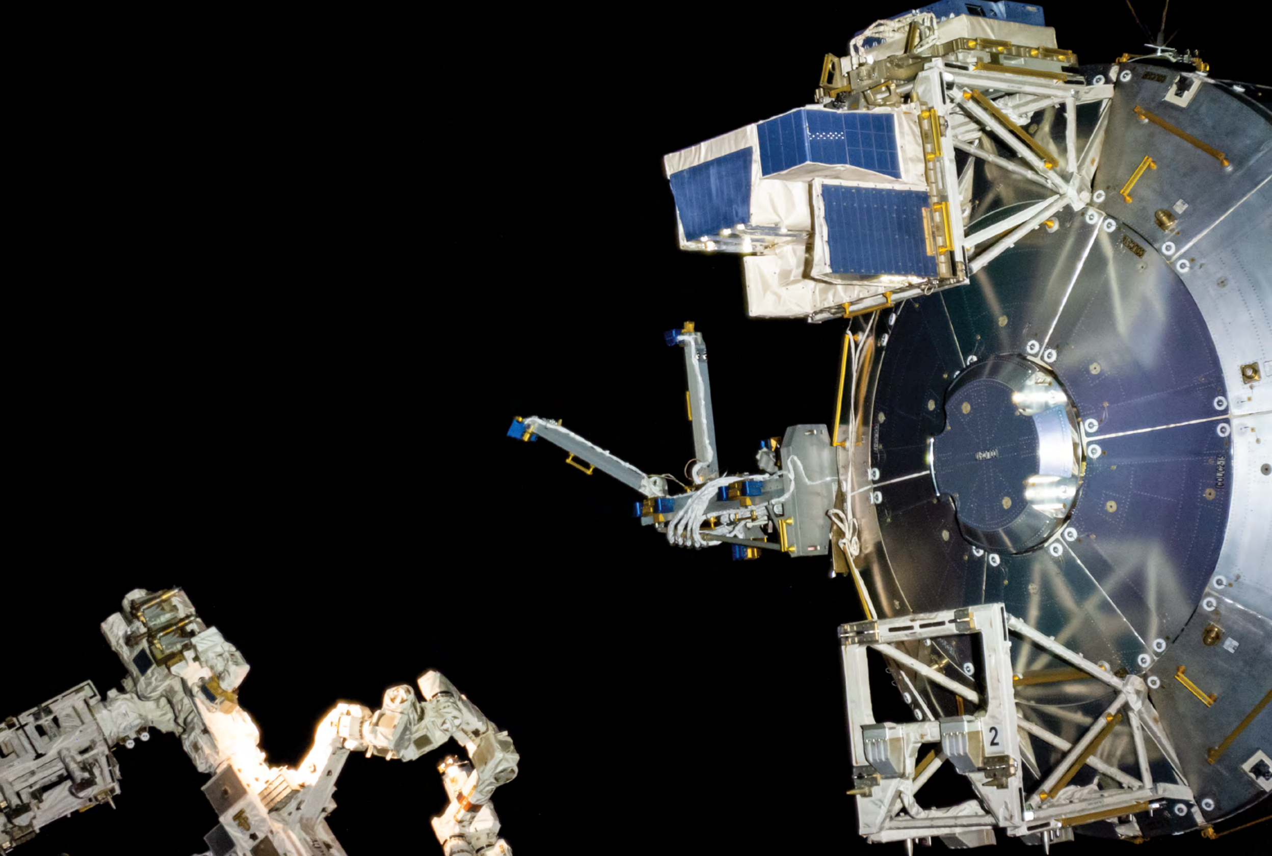
A view of Bartolomeo in its final position on the Columbus module of the International Space Station (ISS). The European external platform Bartolomeo is an enhancement of the ISS European Columbus Module and its infrastructure. Designed to meet user requirements from the commercial and institutional sector, Bartolomeo is a new external payload hosting facility on the ram side of Columbus.
