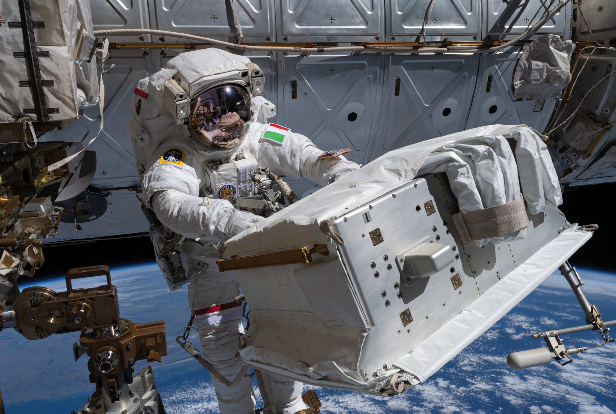
Extravehicular crewmember 1 (EV1) Luca Parmitano, anchored in an Articulating Portable Foot Restraint, holds the Upgraded Tracker Thermal Pump System as he is moved to the Alpha Magnetic Spectrometer worksite. Photo was taken by EV2 during Extravehicular Activity 61.
