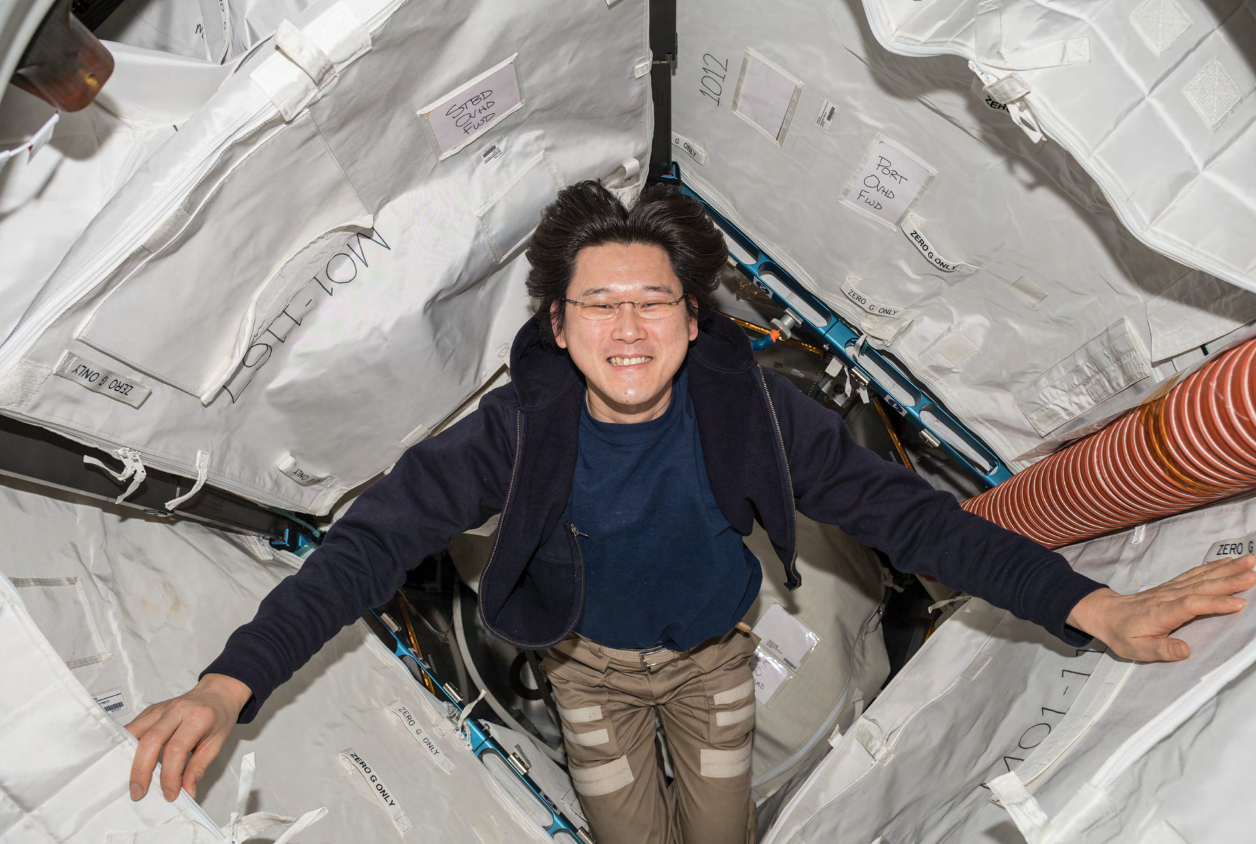
Astronaut Norishige Kanai is photographed inside the Bigelow Expandable Activity Module (BEAM). Future space habitats for low-Earth orbit, the Moon, Mars, or other destinations need to be lightweight and relatively simple to construct. BEAM is an experimental expandable capsule that docks with the International Space Station. After docking, BEAM inflates to roughly 13 feet long and 10.5 feet in diameter to provide a habitable volume where a crew member can enter.
