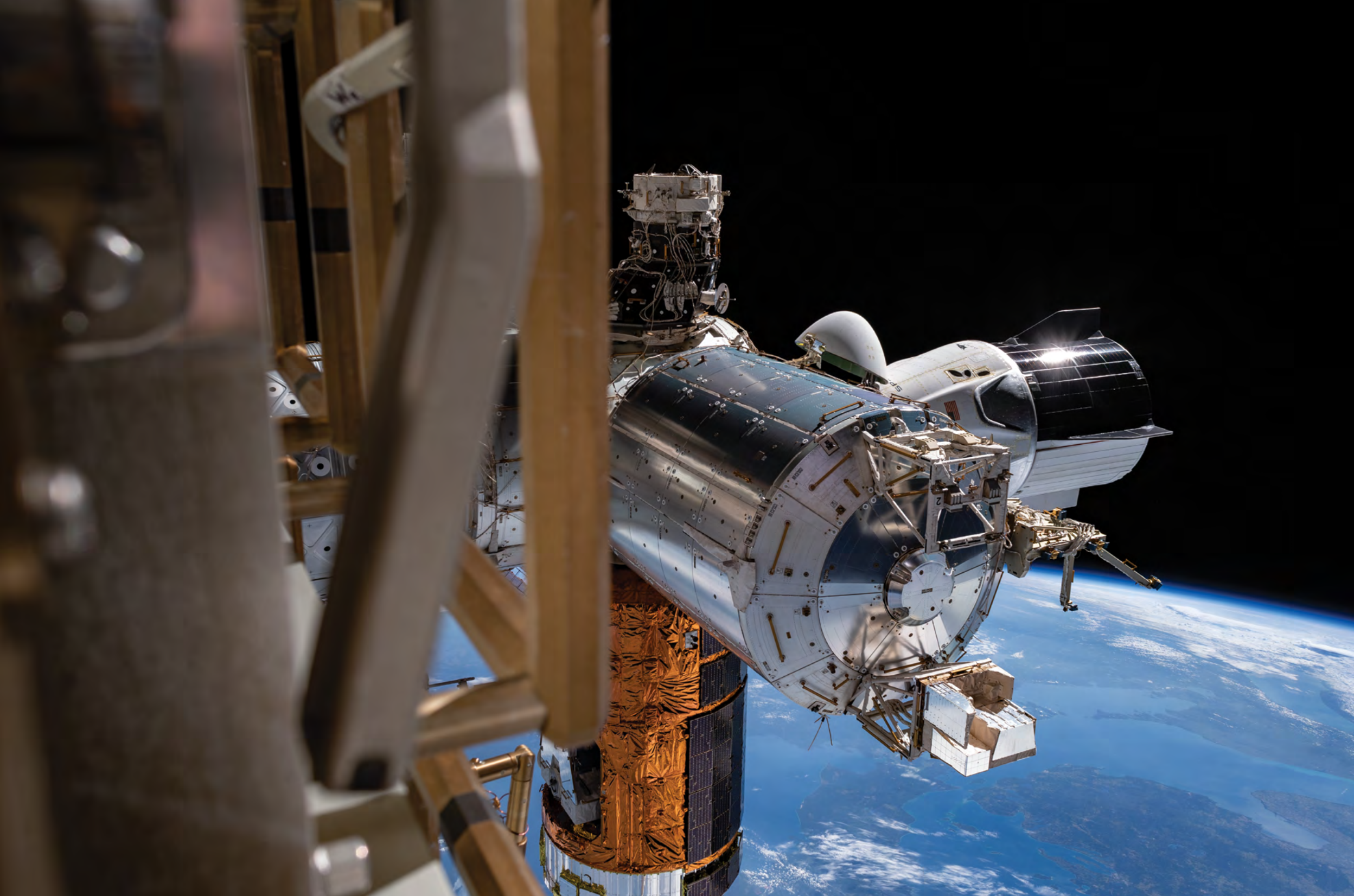
The SpaceX Crew Dragon (center right), the Japanese H-II Transfer Vehicle-9 resupply ship (center bottom) and Europe's Columbus laboratory module figure prominently in this photograph taken during a spacewalk conducted by astronauts Bob Behnken and Chris Cassidy. All three are attached to the U.S. Harmony module with the International Docking Adapter on top.
