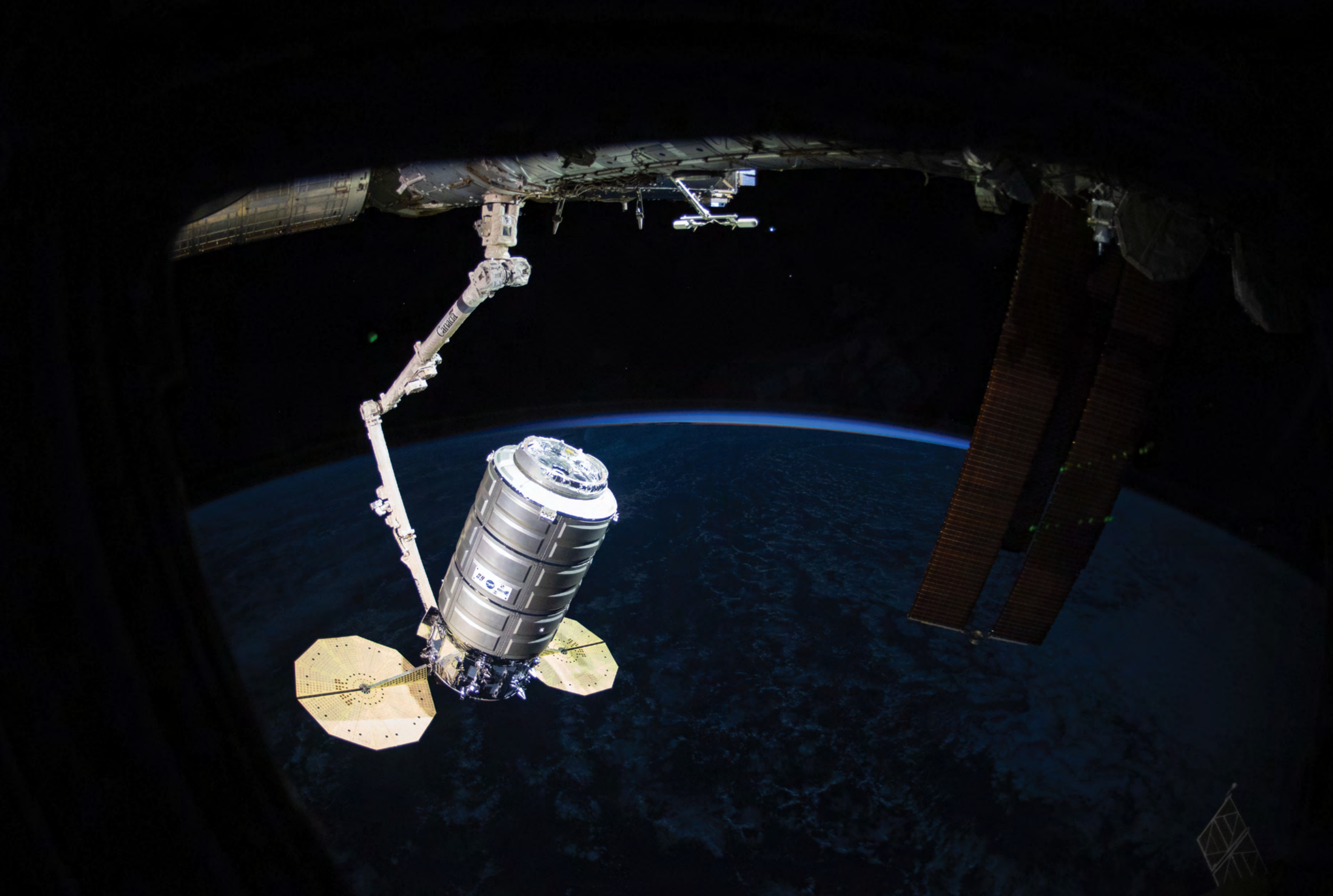
The Space Station Remote Manipulator System Canadarm2 robotic arm grapples the Northrop Grumman Cygnus cargo craft as it approaches its capture point with the International Space Station. Image framed by window.
