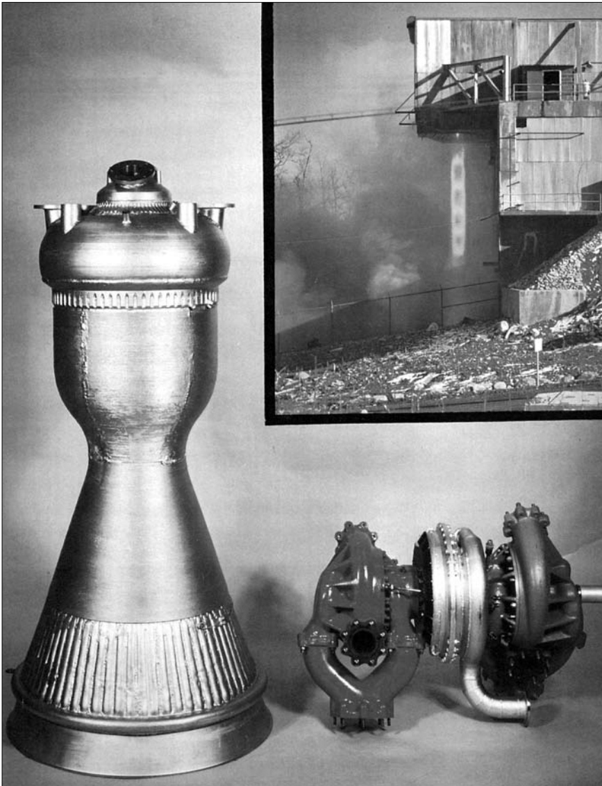
The Reaction Motors XLR30-RM-2 liquid-propellant rocket engine was the leading candidate for the X-15 powerplant. The XLR30 had been developed from the XLR10 that powered the Viking sounding rocket developed for the Naval Research Laboratory. Twelve Vikings were launched between 1949 and 1955. (Reaction Motors Inc.)
