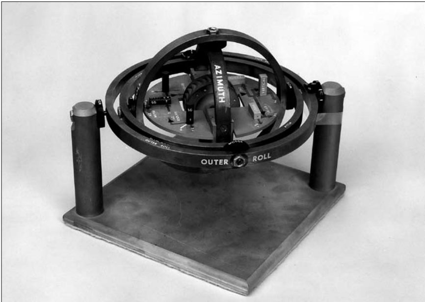
The X-15 was one of the first aircraft to require what is today called an inertial measurement unit, or stable-platform. Gyroscopes of the era were large, heavy, and consumed a considerable amount of power. This model shows the three interlocked rings required to determine position in three dimensions. (NASA)
