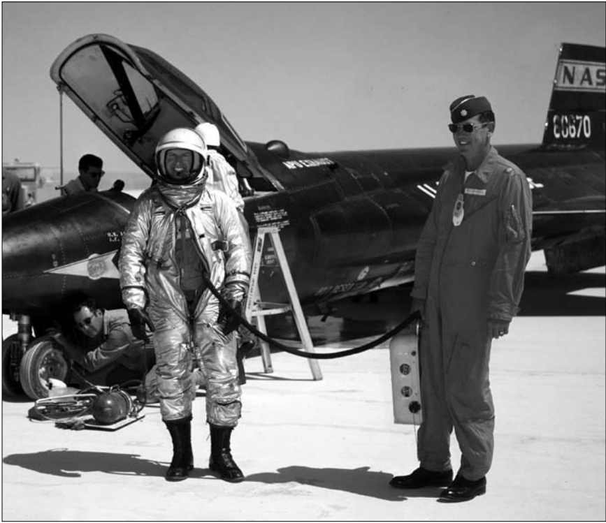
The MC-2 suit led to the David Clark Company A/P22S suit that became the standard military and NASA high-altitude suit. The A/P22S and its variants have had a long career, and were used by SR-71 and U-2 pilots, as well as space shuttle astronauts. Here, NASA test pilot Joseph A. Walker stands in front of an X-15 after a flight. (NASA)
