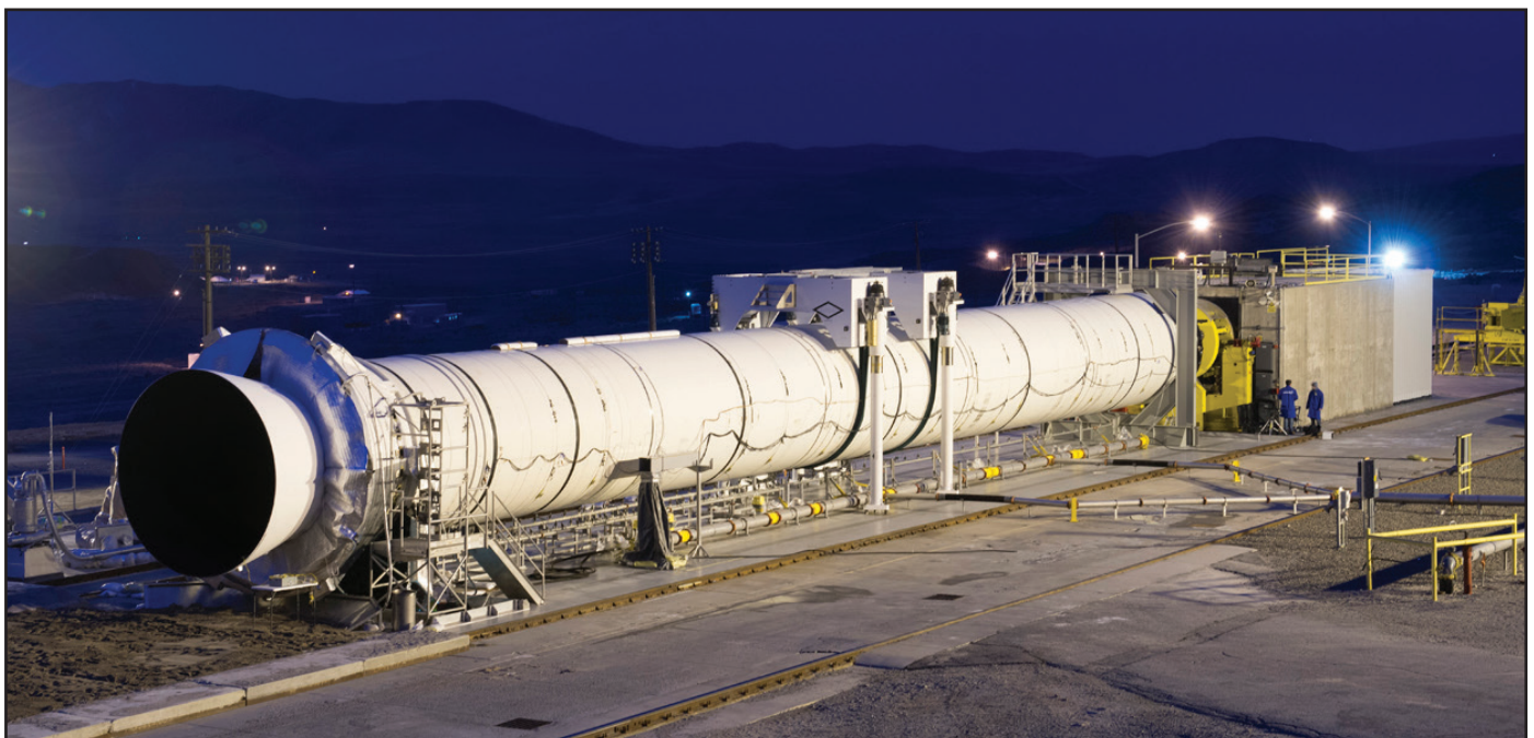
Flight Support Booster (FSB-1) Static Test Firing Northrop Grumman Corporation, Utah. August 2020
