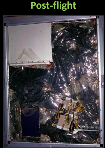
AO erosion of Kapton blanket
