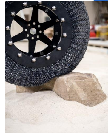
Shape memory alloy (SMA) tires for rovers
