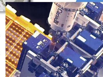
MISSE-FF at ELC-2 Site 3 with the 5 MSCs open
