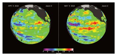
Jason-3 has begun mapping the ocean! This shows sea surface height (blue/magenta indicates lower-than-normal sea levels, while yellow/red indicates higher-than-normal sea levels). Data from Jason-3 will be used to monitor climate change and track phenomena like El Niños.
