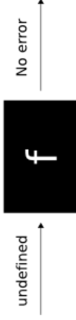
Figure 36 If f returns an error when passed undefined, it must be strict. Otherwise, it's lazy.
