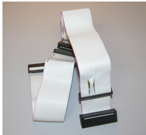
Figure 2.2: Floppy Disk Drive Cable (GFDL, by Shakespeare)
