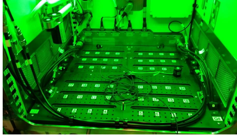
0-100 \mu\text{mol m}^{-2} \text{s}^{-1} at 525 nm \pm 10 nm
